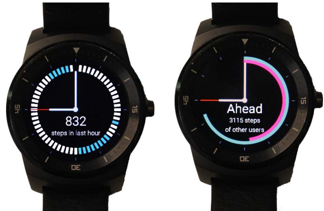
Figure 1 – TickTock (left) and Normly (right), two of the concepts developed as watchfaces. TickTock portrays periods in which one was physically active over the past hour. Normly compares one's goal completion to that of others having a similar walking goal.
